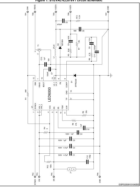
Figure 1: STEVAL-ILL078V1 circuit schematic
