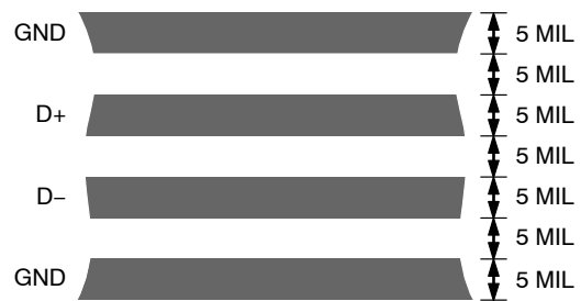
Figure 23. Typical Arrangement of Signal Tracks
