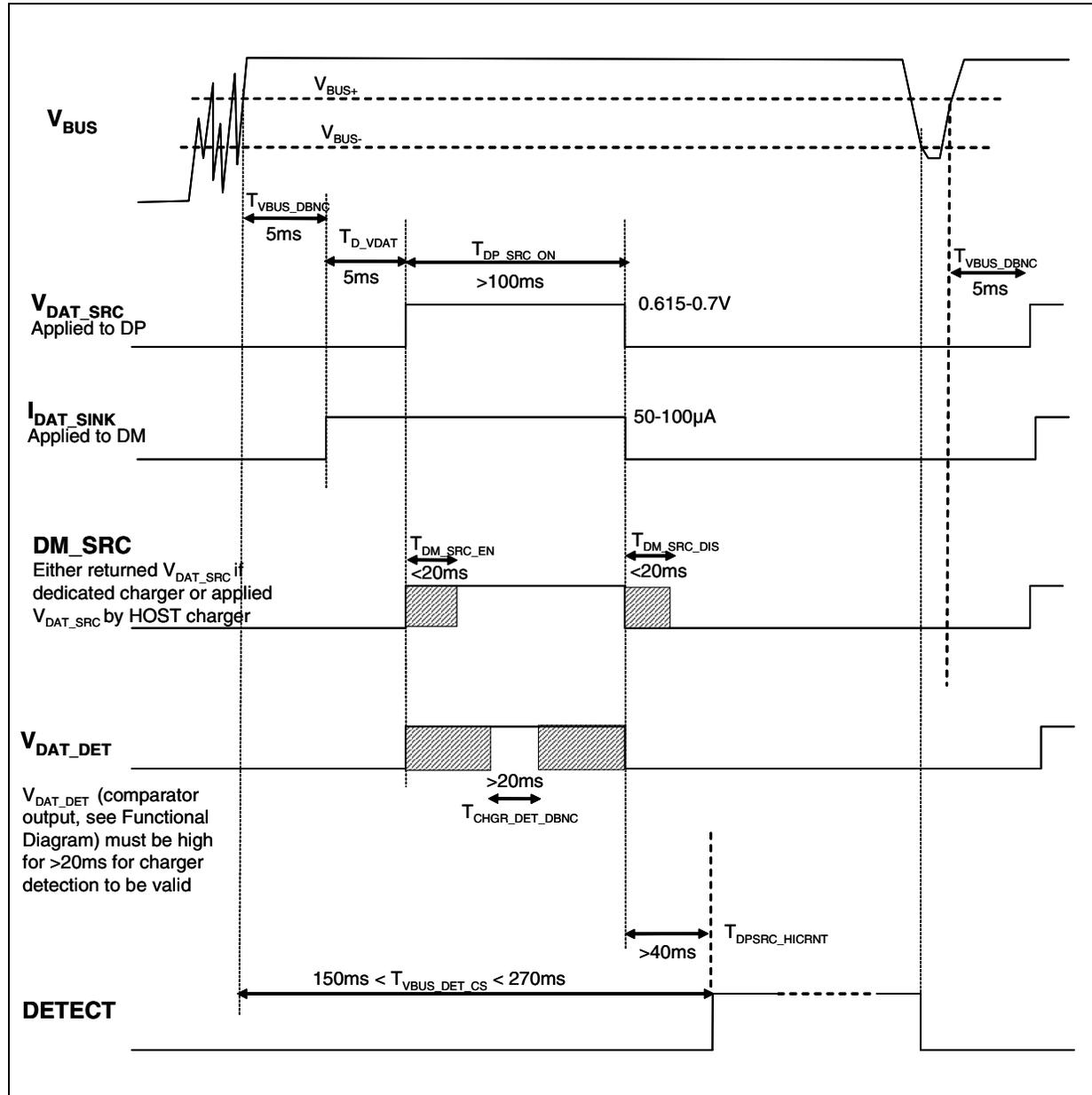
Figure 5. Dedicated charger detection method (with charger connected)
