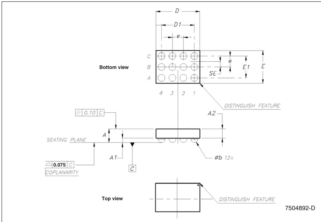
**Tape & reel Flip-Chip 12 mechanical data**
