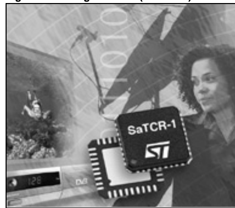
Figure 1. Package: QFN36 (6 x 6 mm)
