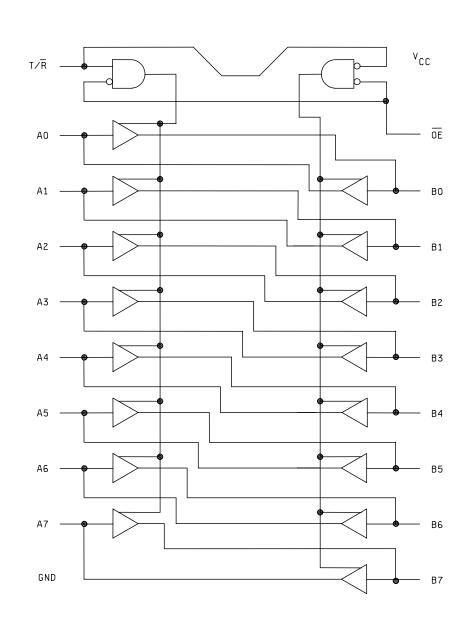
FIGURE 4. Logic diagram.
