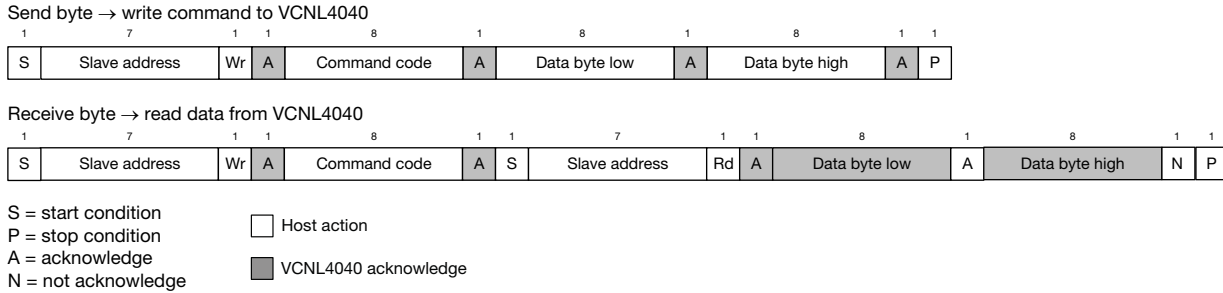
Fig. 12 - Write Word and Read Word Protocol
