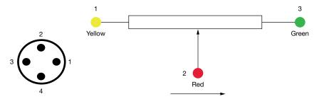
Direction of wiper displacement with shaft extended
