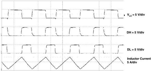
1 \mu\text{s/div} V_{IN} = 5 \text{ V} , V_{OUT} = 2.5 \text{ V} , Load Current = 5 A, L = 1.5 \mu\text{H} , C_{OUT} = 220 \mu\text{F} \times 2 Typical Switching Waveform
