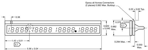
5.1 > Fill tube is concentric with hole within ± 0.060 vertically and + 0.060/- 0.030 horizontally.
