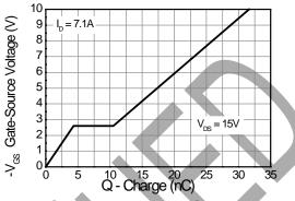
Gate-Source Voltage v Gate Charge
