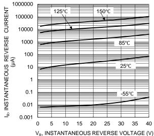
V<sub>R</sub>, INSTANTANEOUS REVERSE VOLTAGE (V Figure 2. Typical Reverse Characteristics
