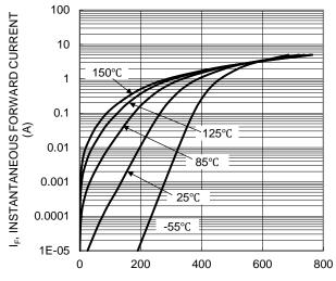
V<sub>F</sub>, INSTANTANEOUS FORWARD VOLTAGE (mV) Figure 1. Typical Forward Characteristics
