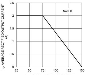
T<sub>A</sub>, AMBIENT TEMPERATURE (°C) Figure 3. DC Forward Current Derating Curve
