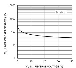
Figure 5. Typical Junction Capacitance
