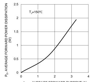
I<sub>F(AV)</sub>, AVERAGE FORWARD CURRENT (A) Figure 4. Forward Power Dissipation
