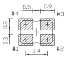
\*External high-frequency power decoupling is recommended.(see test circuit for minimum recommendation). To ensure optimal performance, do not route traces beneath the package.
