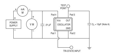
Note A: CL includes probe and jig capacitance.
