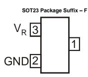
(Top View) Pin 1 should be left floating or Connected to Pin 2
