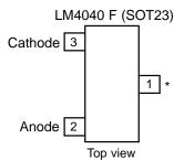
\* Pin 1 must be left floating or connected to pin 2
