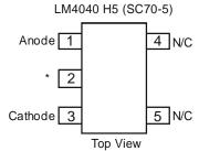
\* Pin 2 must be left floating or connected to pin 1
