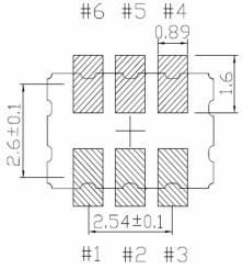
\*External high-frequency power decoupling is recommended.(see test circuit for minimum recommendation). To ensure optimal performance, do not route traces beneath the package.
