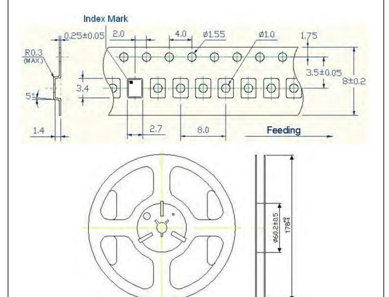
1. 230mm minimum leafer which consist of carrier and/or tape followed by a minimum of 160mm of empty carrier tape sealed with cover tape.
