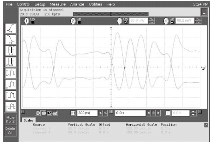
Data Waveforms, 3.0Gbps (left) & 6.0Gbps (right)
