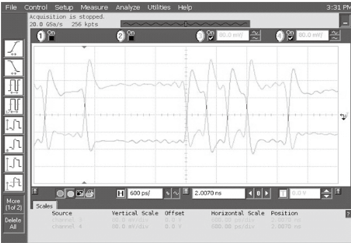
Data Waveforms, 3.0Gbps (left) & 6.0Gbps (right)
