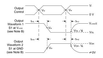
Voltage Waveform Enable and Disable Times Low and High Level Enabling
