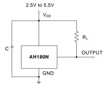
Note: C is for power stabilization and to strengthen the noise immunity, the recommended capacitance is  $10nF \sim 100nF$ . R<sub>L</sub> is the pull-up resistor, the recommended resistance is  $10kOhm \sim 100kOhm$ .
