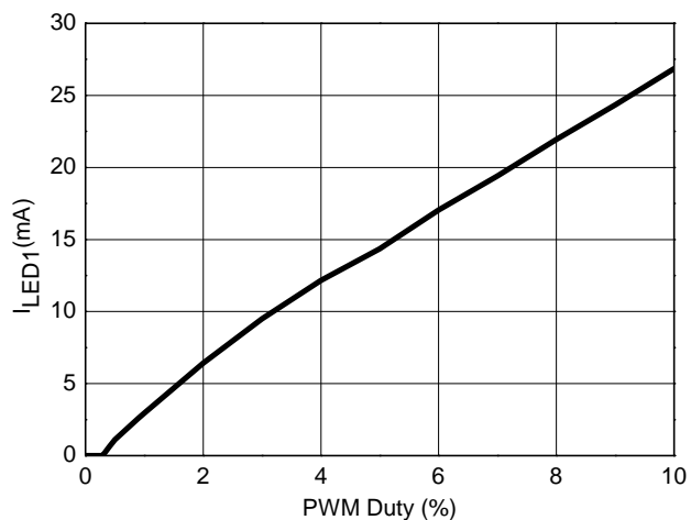
LED Current (AL1782) vs. PWM Duty (f=500Hz, 0~10%)
