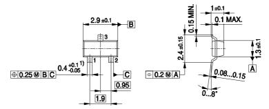
1) Lead width can be 0.6 max. in dambar area
