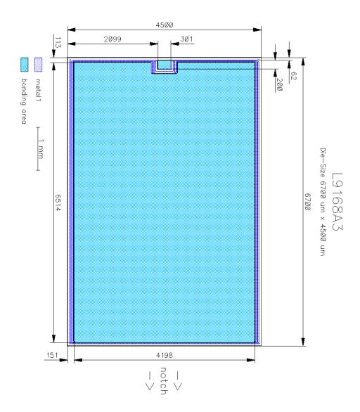
Figure 1 Outline Chip, dimensions in µm
