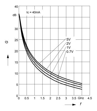
Power gain  $G_{ma}$ ,  $G_{ms} = f(I_C)$  $V_{CE} = 3V$
