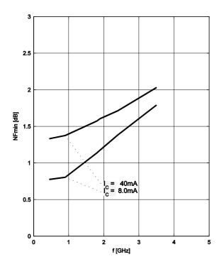
Noise figure  $F = f(I_C)$  $V_{CE} = 3V, f = 1.8 \text{ GHz}$
