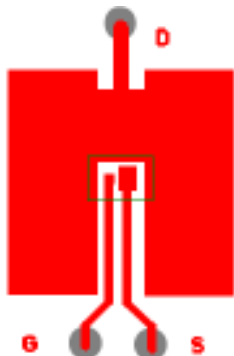
⑥ Surface mounted on 1 in. square Cu board (still air).
