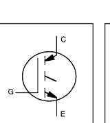
600 V  $I_{C(nom)} = 12A$ V<sub>CE(on)</sub> typ. = 1.55V @ I<sub>C(nom)</sub> @ 25°C Motor Control IGBT Short Circuit Rated 150mm Wafer
