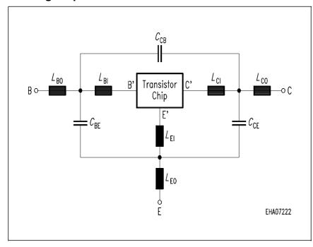
0.84 nΗ 0.51  $L_{\mathsf{BO}} =$ nΗ 0.69 nΗ 0.61 nΗ  $L_{CI} =$ 0 nΗ  $L_{CO} =$ 0.49 nΗ  $C_{\mathsf{BE}} =$ fF 84  $C_{CB} =$ fF 165  $C_{CE} =$ fF Valid up to 6GHz
