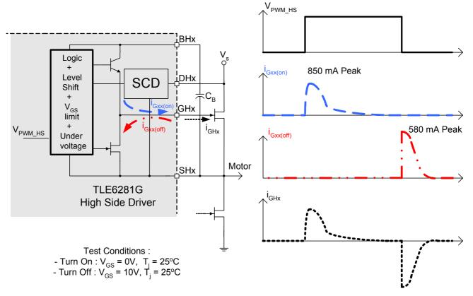
This figure represents the simplified internal circuit of one high side gate drive. The drive circuit for the low sides looks similar.
