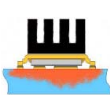
⑤ Mounted to a PCB with small clip heatsink (still air)
