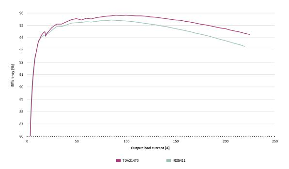
Efficiency levels at f<sub>sw</sub> = 500 kHz, V<sub>in</sub> = 12 V, V<sub>out</sub> = 1.82 V, five-phase measurement
