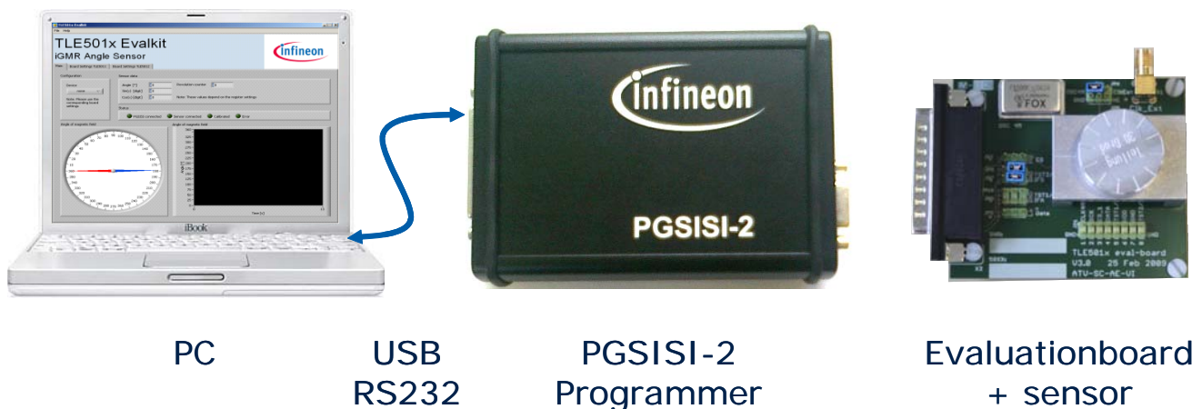
Figure 1 Tool configuration for evaluation of hall sensors with PGSISI-2
