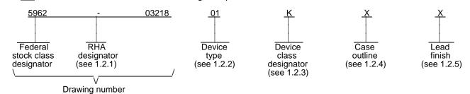
1.2.1 <u>Radiation hardness assurance (RHA) designator</u>. RHA marked devices shall meet the MIL-PRF-38534 specified RHA levels and shall be marked with the appropriate RHA designator. A dash (-) indicates a non-RHA device.
