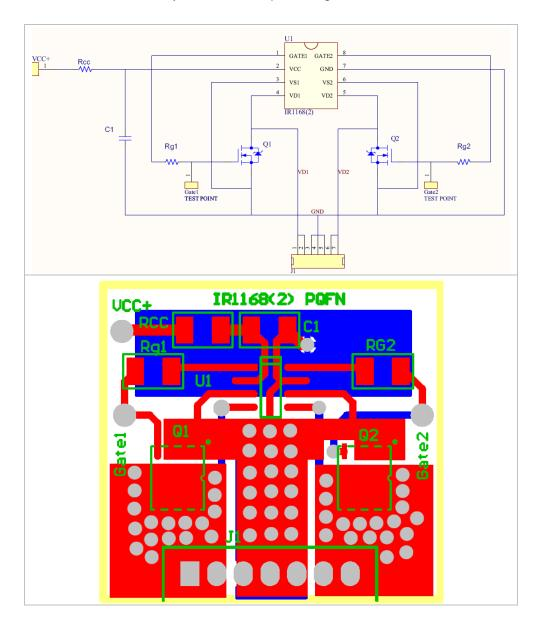
The daughter card shown above is designed to allow easy retrofit in existing systems with minimal system changes. This PQFN daughter card can carry 10A output current with  $8m\Omega$  Rdson MOSFET.
