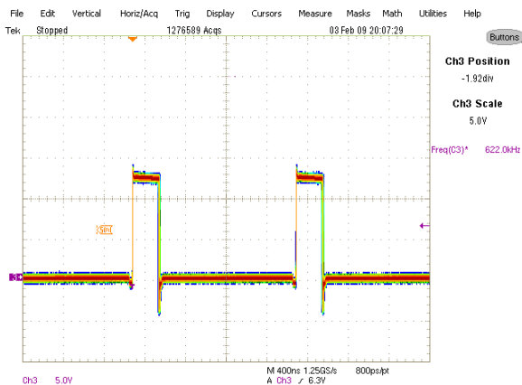
Fig. 11: Inductor node at 8A load Ch 3 :LX
