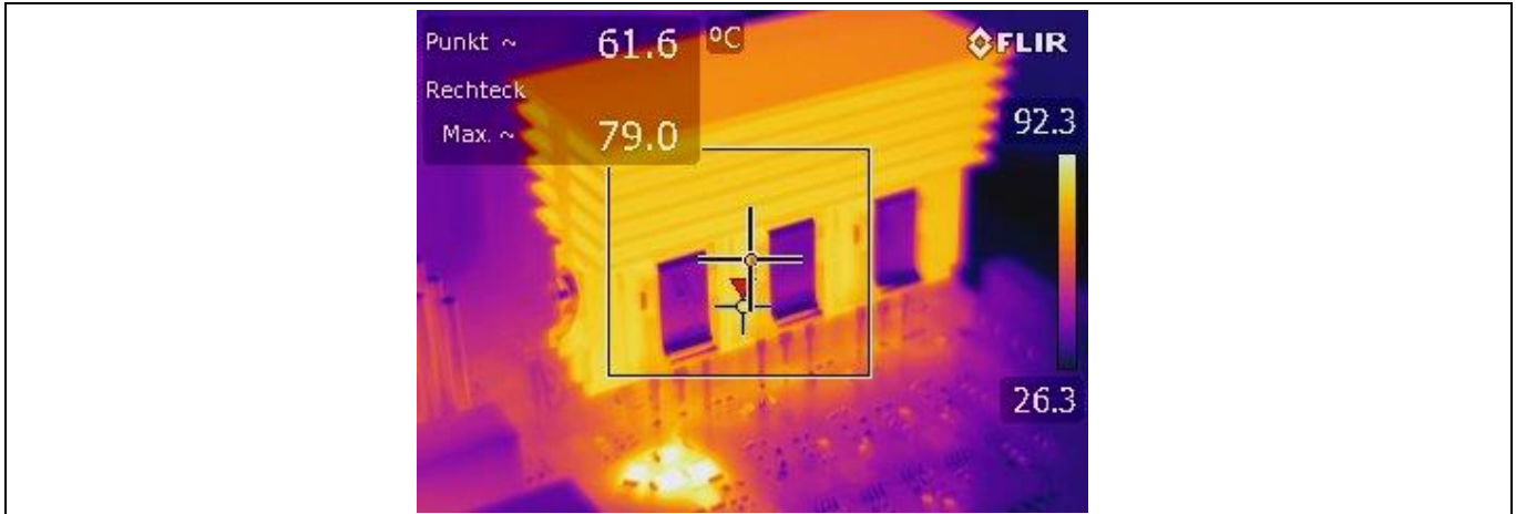
Figure 30 Thermal image the left power MOSFETs
