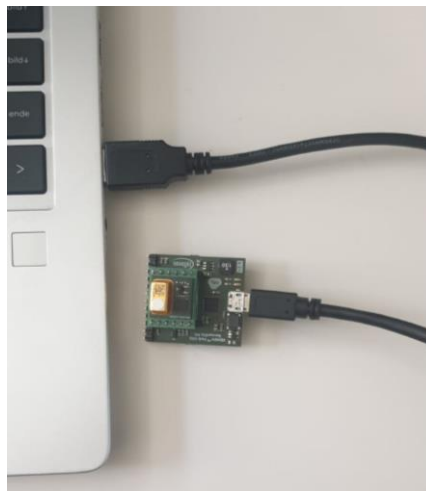
Figure 6 XENSIV™ PAS CO2 Sensor2Go Evaluation kit connection to PC via micro USB cable
