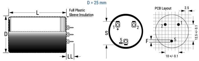
Connections: Hole 1 represents +ve. Hole 5 Represents -ve. Terminals 2,3, and 4 may be at negative terminal potential due to the presence of electrolyte. They are intended for mechanical connections only. It is recommended that they are soldered to the printed cicuit board. Additional dummy pins are provided for stability. Note that the case and dummy pins may be at negavtive terminal potential
