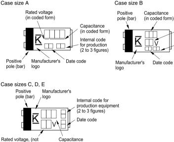
Rated voltage, (not coded)  $V_R = 6.3 V$ is abbreviated as 6.
