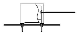
Temperature monitored inside the capacitor.
