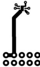
d. 151\text{ }^\circ\text{C/W} when mounted on a minimum pad of 2 oz copper
