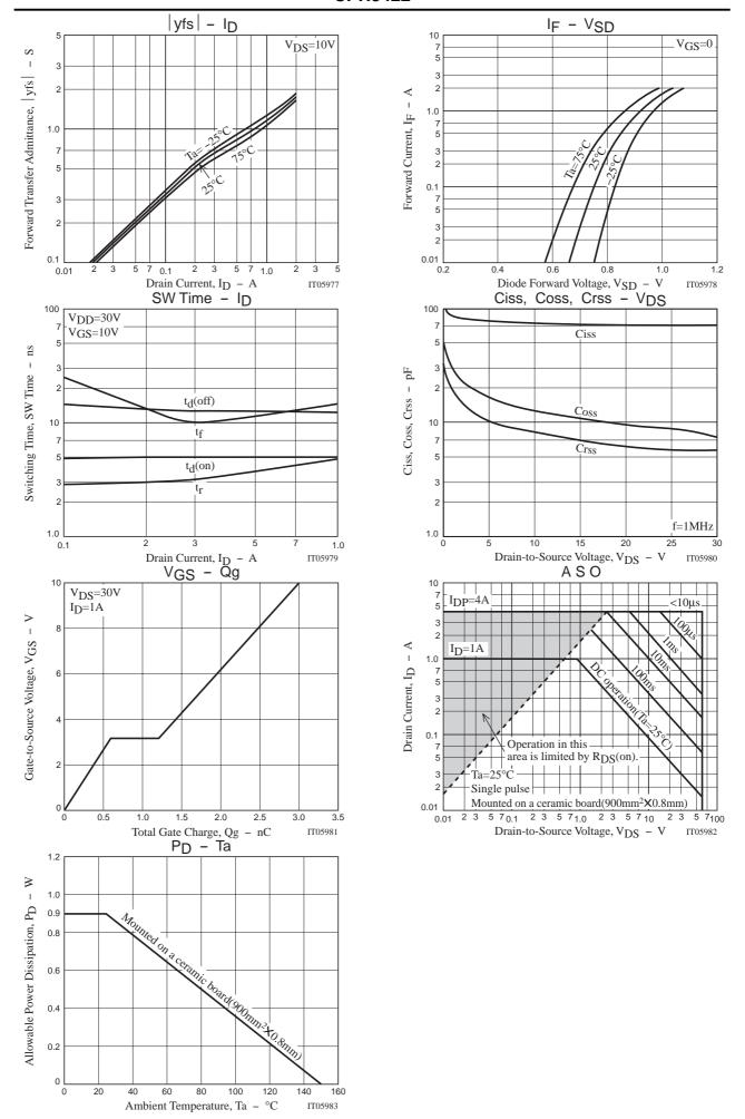
Note on usage: Since the CPH3422 is designed for high-speed switching applications, please avoid using this device in the vicinity of highly charged objects.
