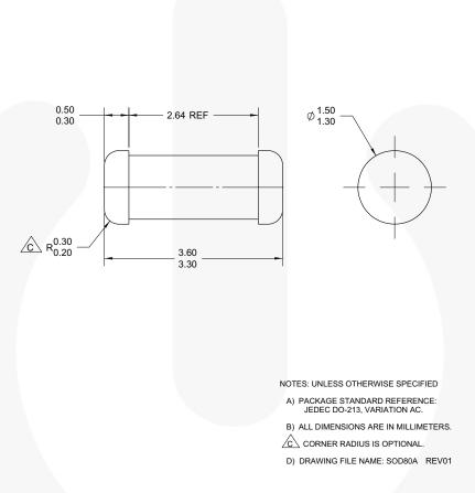
Figure 11. 2-TERMINAL, SOD-80, JEDEC DO-213AC, MINI-MELF
