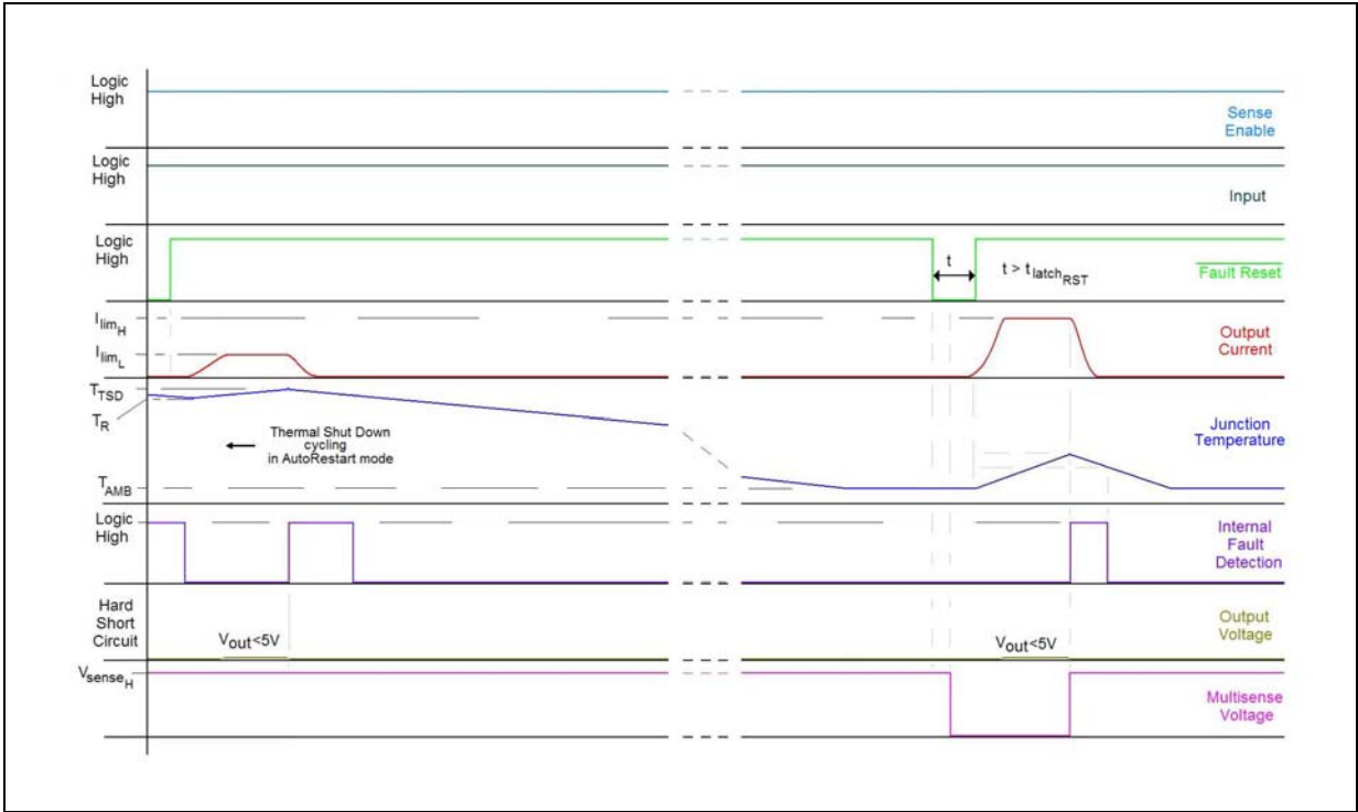
Figure 11. Latch functionality - behavior in hard short circuit condition
