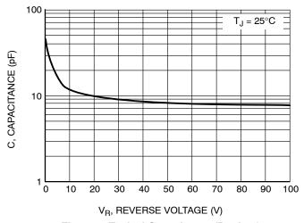
Figure 6. Typical Capacitance (Per Leg)
