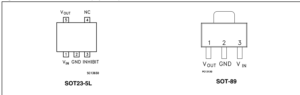
Figure 2. Pin connections (top view)
