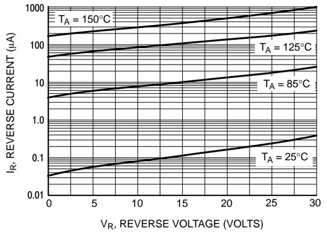
**Figure 3. Leakage Current**
