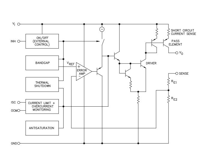
FIGURE 3. Block diagram.
