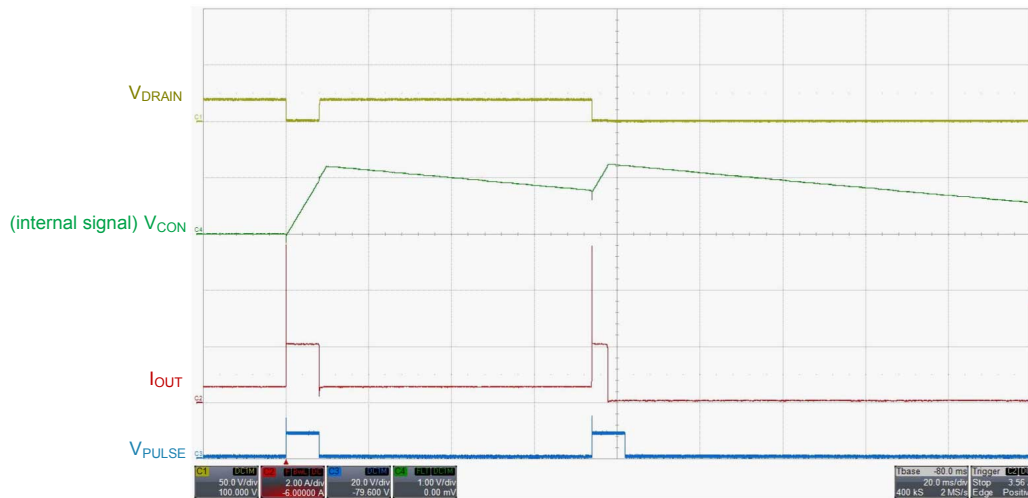
Figure 8. Behavior under repetitive overloads (magnification)
