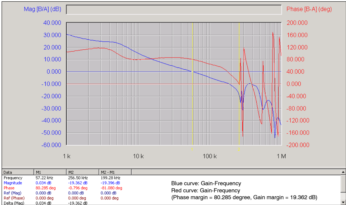
Figure 14. Closed-loop Voltage Loop-gain of the NCP1587
