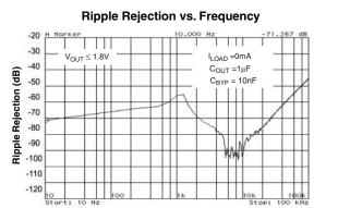
**Ripple Rejection vs. Frequency**
